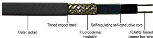
PLSRS self-regulating pipe trace cable.
