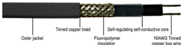
PLSRS self-regulating pipe trace cable.
