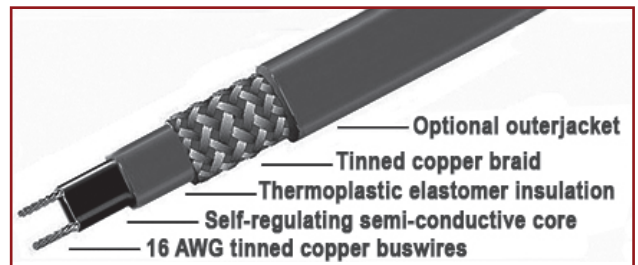
Cutaway view of ProLine self-regulating heat cable.
