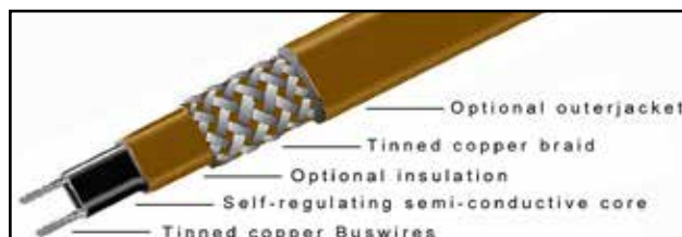
Cutaway view of PLSRP self-regulating heat trace cable.
