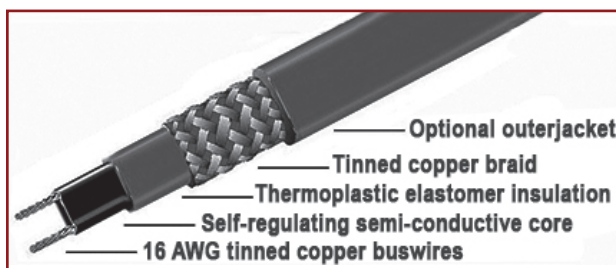
Cutaway view of ProLine self-regulating heat cable.
