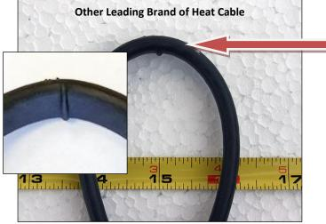
Other cable "bubbles" and pulls away from the core at a typical bend radius of 2 inches.
